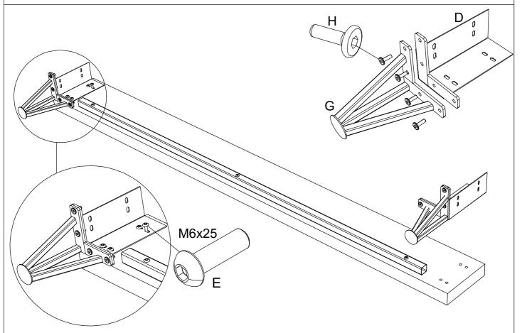
Use the screw shown above to attach the corner bracket to the side panels and footboard panels of the bed frame.
